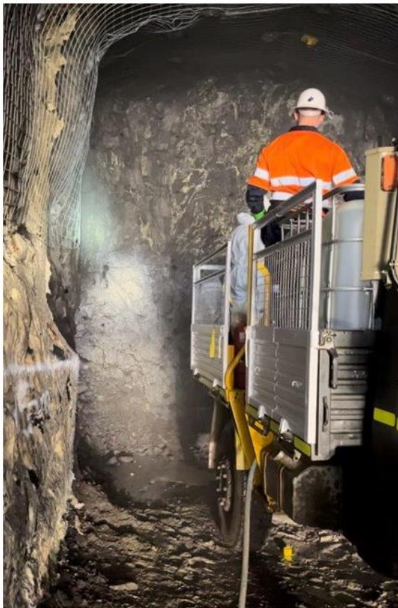
Figure 6 Securing the face with thin spray-on liner (LHS) and Figure 7 part of the ROM stockpile(RHS)
